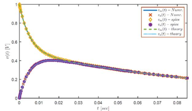
Figure 7: Comparing the evolution of  $v_m(t)$  and  $v_s(t)$  according to Matlab, SPICE and the theoretical calculation given by equations (12) and (13) respectively. At time  $t = 0$ ,  $v_m(t) = v_{m_0} = 1V$ ,  $v_s(t) = 0V$ ,  $q_0 = 0.3q_d$ ,  $R = 100K\Omega$ ,  $C = 1\mu F$ ,  $R_{off} = 16K\Omega$  and  $R_{on} = 100\Omega$ .
