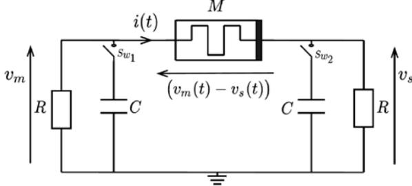
Figure 6: Two pixel cells system composed of master and a slave cells coupled together by a memristor, with the cell parameters given by the subscripts  $m$  and  $s$  respectively.  $M$  is the memristor whose model is given by equation (4).
