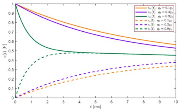
Figure 8: The evolution of  $v_m(t)$  and  $v_s(t)$  for  $q_0 = 0.1q_d$ ,  $0.3q_d$  and  $0.9q_d$  respectively. At  $t = 0$ ,  $v(t) = v_{m_0} = 1V$ ,  $v(t) = 0V$ ,  $R = 100K\Omega$ ,  $C = 1\mu F$ ,  $R_{off} = 16K\Omega$  and  $R_{on} = 100\Omega$ . The result showed the effect of  $M(q_0)$  on the dynamics toward the steady state.
