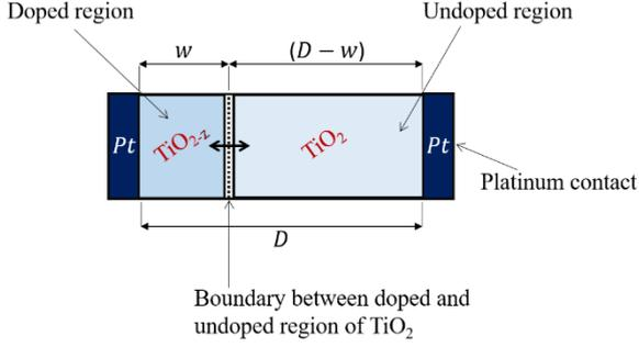
Figure 4: Structure of  $\text{TiO}_2$  memristor.  $D$  is the width of the entire sandwiched  $\text{TiO}_2$  layer,  $w$  is the width of doped  $\text{TiO}_{2-x}$  and  $D-w$  is the width of the undoped  $\text{TiO}_2$ , so the equivalent memristance is:  $M(w) = R_{on} \frac{w}{D} + R_{off} \left(1 - \frac{w}{D}\right)$ .
