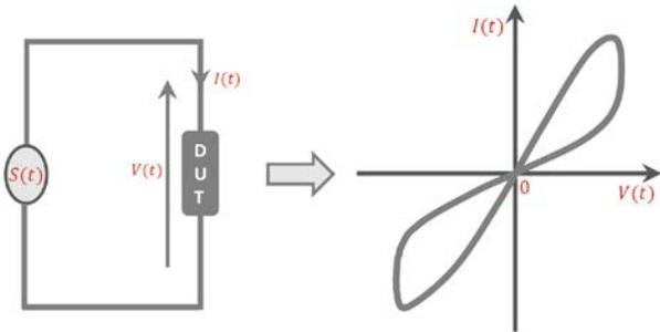
Figure 3: Memristor device under test (D.U.T) as a black box (left) and Current-voltage response of the black box (right).  $S(t)$  is the periodic input source and it could be a voltage or a current source.
