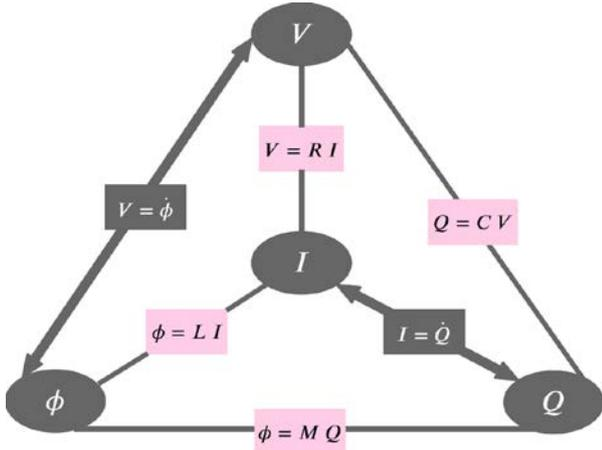
Figure 2: Symmetrical argument of the four basic passive circuit elements with respect to the four circuit variables.
